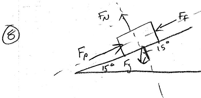
$$\begin{aligned} \text{x} \\ \sum F &= 0 \\ F_p - F_f - F_g \sin 15 &= 0 \\ F_p - F_f - mg \sin 15 &= 0 \\ F_p - (141.99) - 60(9.8) \sin 15 &= 0 \end{aligned}$$
