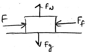
$$\begin{aligned} F &= F_f \\ F_f &= 50 \text{ N} \end{aligned}$$
